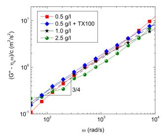
Figure 2. Determination of the persistence length from high frequency oscillatory squeeze flow measurements. The reduced linear viscoelastic loss modulus  $G''-\omega\eta_s$  measured by squeeze flow normalized by concentration as a function of frequency  $\omega$ . The dashed line represents a fit with a slope of  $^3/_4$ , which results in of  $I_p = 0.65 \pm 0.1~\mu m$  using equation (2). doi:10.1371/journal.pone.0093194.g002
