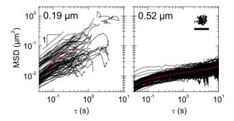
Figure 1. Determination of the mesh size by multiple particle tracking. MSDs against time  $\tau$  and the individual trajectories after  $\tau=3$  s (inset) of microspheres with diameters of 0.19 and 0.52  $\mu$ m at a K8/K18 concentration of 1.0 g/l (19.7  $\mu$ M). The scale bar for the trajectory shown in the right panel denotes 500 nm and is the same in both panels and directions. The red line represents the average MSD. doi:10.1371/journal.pone.0093194.g001
