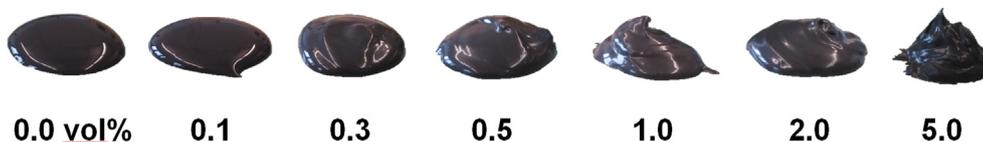
**Fig. 7.** Characteristic texture of anode slurries ( $\phi_{\text{total}} = 20 \text{ vol}\%$ : graphite, CB and CMC in water; the ratio of graphite to CB to CMC is 95.4:2.0:2.6) with different amounts of secondary fluid octanol as indicated above.
